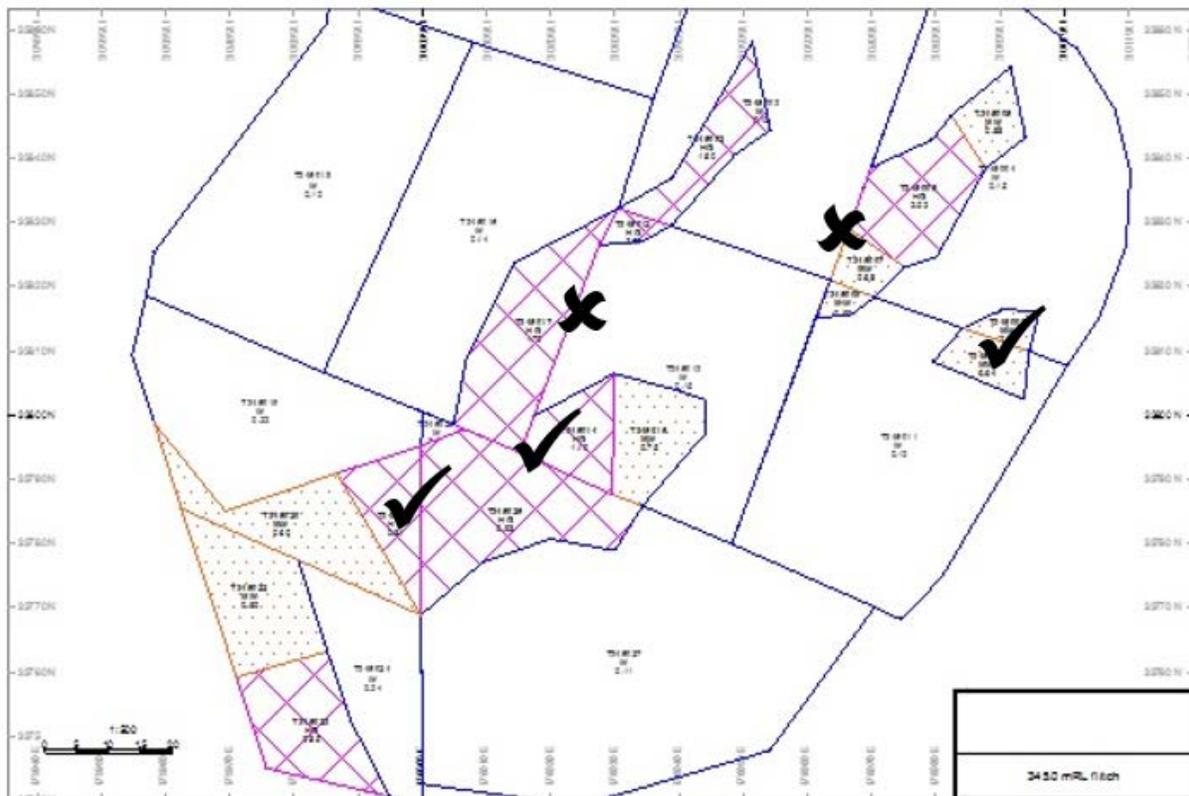
Ideally mineralisation wireframes should be built as mining progresses, and be based on the existing resource wireframes adjusted for the closer spaced GC data in order to create your dig blocks.
