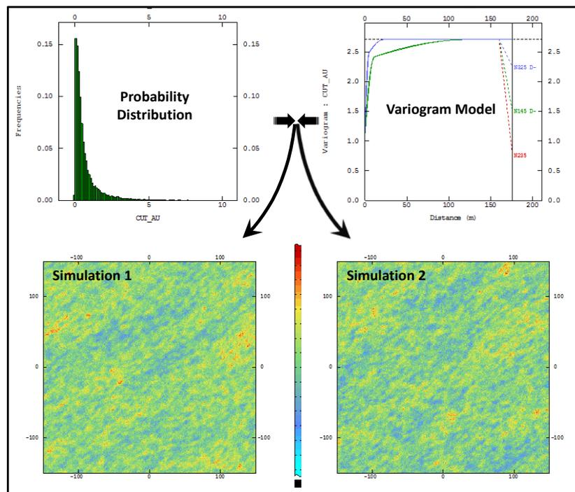
Figure 1: Two simulated realisations which have reproduced the same input distribution and input variogram.
