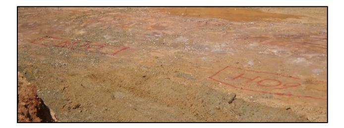
When creating dig blocks, use all available information, including data from the bench above (previous GC drilling) and below (resource or deeper GC drilling) and data across individual blasts. The diagram below shows examples where adjacent blasts were considered (good) and not considered (bad), when creating dig blocks.
